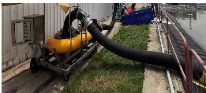
Fig. 4 Shrimp harvesting machine with impeller model IM3 (size 254 mm)
