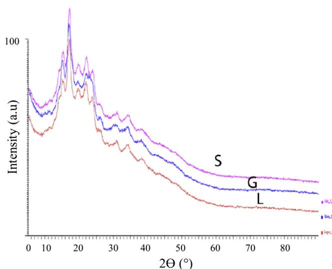
**Fig. 1.** X-ray powder diffraction patterns of Lagos (L), Giwa (G) and Sule (S) starches.
