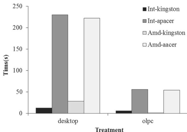
Fig. 6. Boot time for desktop computer compared to “One Laptop per Child” (OLPC) computer for four different computer and storage type configurations (int-kingston, int-apacer, amd-kingston and amd-apacer).
