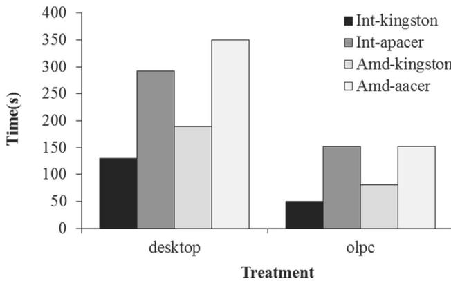
Fig. 2. Mean ping time for desktop computer compared to “One Laptop per Child” (OLPC) computer for four different computer and storage type configurations (int-kingston, int-apacer, amd-kingston and amd-apacer).
