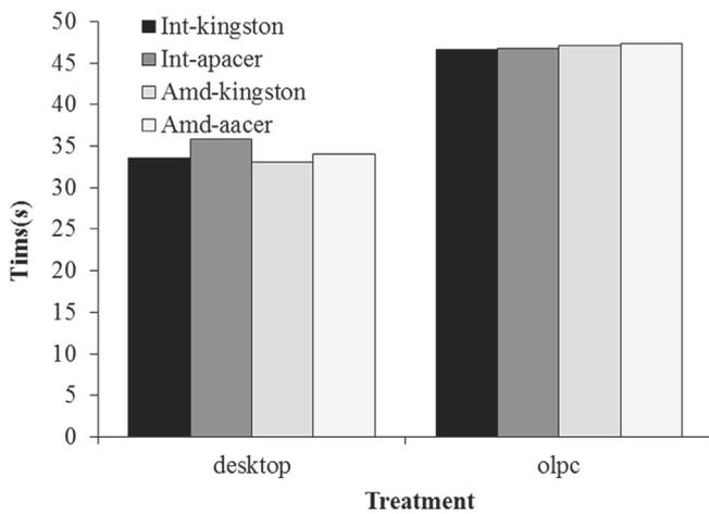
Fig. 1. Mean boot time for desktop computer compared to “One Laptop per Child” (OLPC) computer for four different computer and storage type configurations (int-kingston, int-apacer, amd-kingston and amd-apacer).
