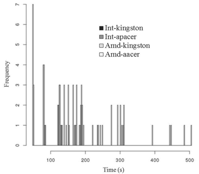
Fig. 3. Histogram of boot time for four different computer and storage type configurations (int-kingston, int-apacer, amd-kingston and amd-apacer).
