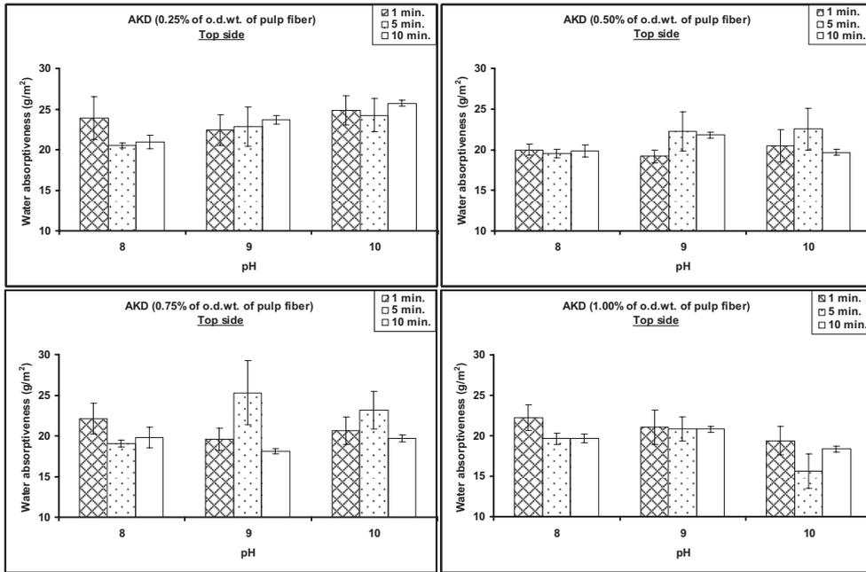
**Figure 1** Effect of changes in AKD dosage (as % of o.d. wt. of pulp fiber) on water absorptiveness of the top side of handsheets at various pH levels of pulp suspension, and mixing times (min). Bars = 95% confidence interval.
