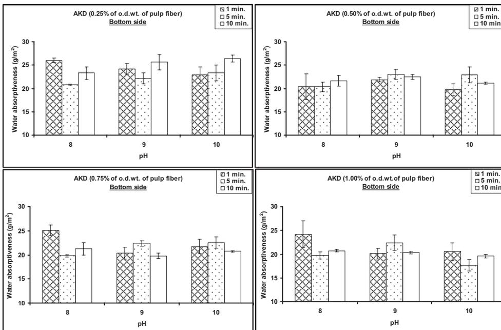
**Figure 2** Effect of changes in AKD dosage (as % of o.d. wt. of pulp fiber) on water absorptiveness of the bottom side of handsheets at various pH levels of pulp suspension, and mixing times (min). Bars = 95% confidence interval.
